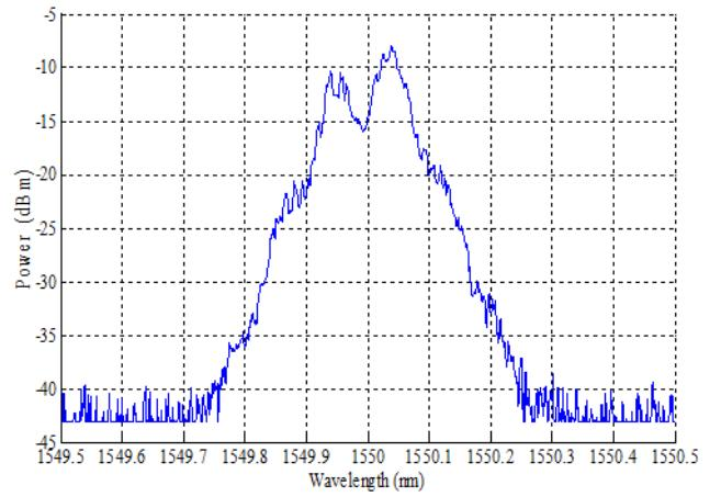
**Figure 5.** OSA displays the output of the system shown in Figure 4 (Laser Power 15mW, Fiber loop mirror length 6.6 Km and OSA Resolution 0.07 nm)
