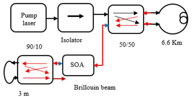
**Figure 4.** Brillouin beam generation using double fiber loop mirror.
