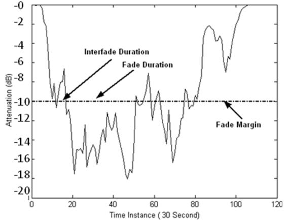
Figure 1: Typical rain attenuation occurring in India at 30 GHz.
