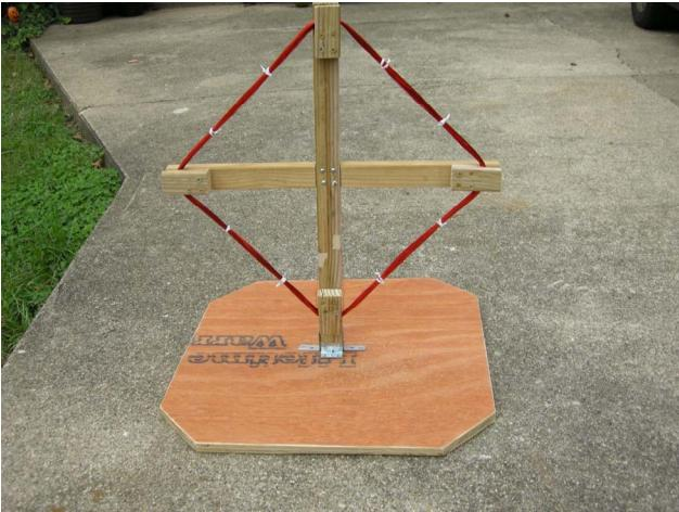
Figure 3. The loop antenna.
