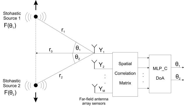
**Figure 1.** Angular position of mobile stochastic EM sources with different signal levels with respect to the sensors of antenna array performing the sampling of the received signals
