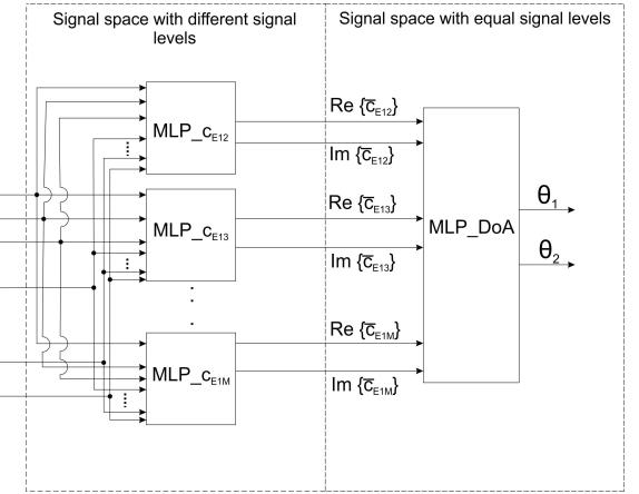
**Figure 2.** Architecture of the two-stage cascade neural model (MLP\_C)
