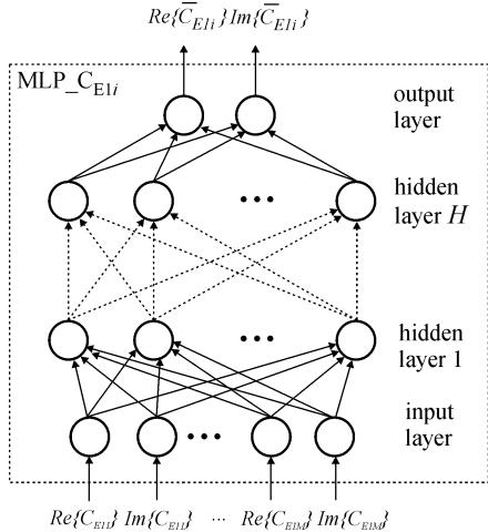
**Figure 3.** MLP architecture used in  $\text{MLP}_{C_{1m}}$  and  $\text{MLP}_{\text{DoA}}$  networks
