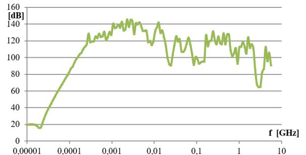
**Figure 5. FN 700Z-20-03 filter attenuation in the frequency range of 150 kHz – 30 MHz**
