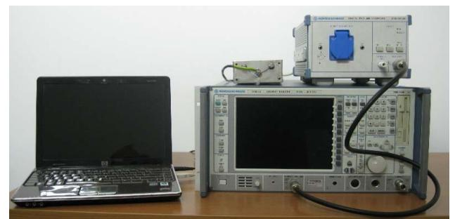
**Figure 4. Illustration of a measurement system designed to measure conducted noise**
