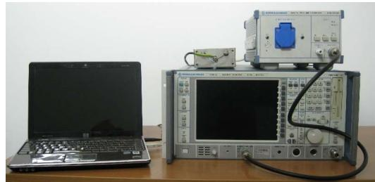
**Figure 2. Illustration of a measurement system designed to measure conducted noise levels**
