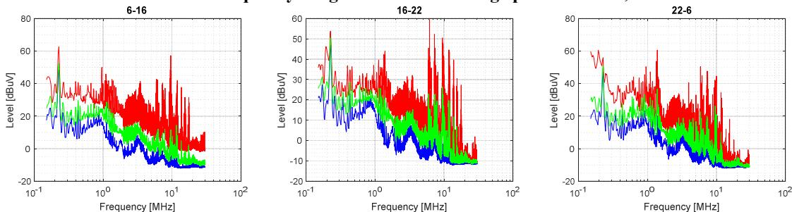
**Figure 6 Maximum (red), minimum (blue) and average (green) values for the conducted background noise level  $U_{n,b}$  measured in the 150 kHz – 30 MHz frequency range on all low voltage power lines:  $L_1$ ,  $L_2$ ,  $L_3$  and  $N$  for a rural area measured during the day (from 6 AM to 4 PM), the evening (from 4 PM to 10 PM) and during the night (from 10 PM to 6 AM)**
