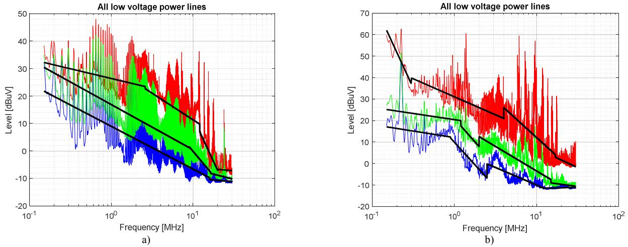
**Figure 7 Maximum (red), minimum (blue) and average (green) values along with approximation functions for the conducted background noise level  $U_{n,b}$  measured in the 150 kHz – 30 MHz frequency range on all low voltage power lines:  $L_1, L_2, L_3$  and  $N$  in: a) an urban area over a 24-hour period, b) a rural area over a 24-hour period**
