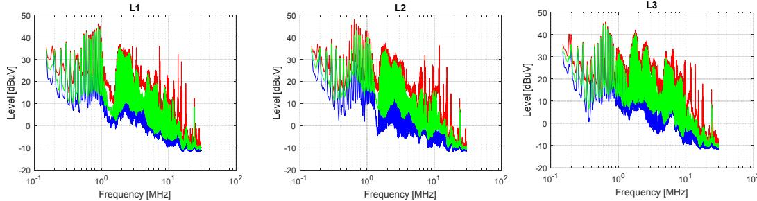
**Figure 3. Maximum (red), minimum (blue) and average (green) values for the conducted background noise level  $U_{n,b}$  measured in the 150 kHz – 30 MHz frequency range on each low voltage power line:  $L_1$ ,  $L_2$  and  $L_3$  in an urban area**
