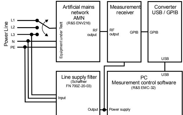
**Figure 1. Block diagram of a measurement system designed to measure conducted background noise voltage levels  $U_{n,b}$  for a frequency range of 150 kHz - 30 MHz**
