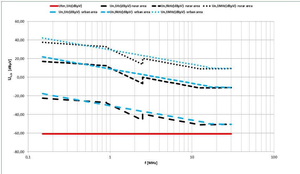
**Figure 8. Functions approximating minimum voltage levels for conducted environment noise in low voltage power lines, in a frequency range of 150 kHz – 30 MHz for band  $b=1$  Hz, 9 kHz and 1 MHz, for various frequency ranges and for each type of measurement location.**
