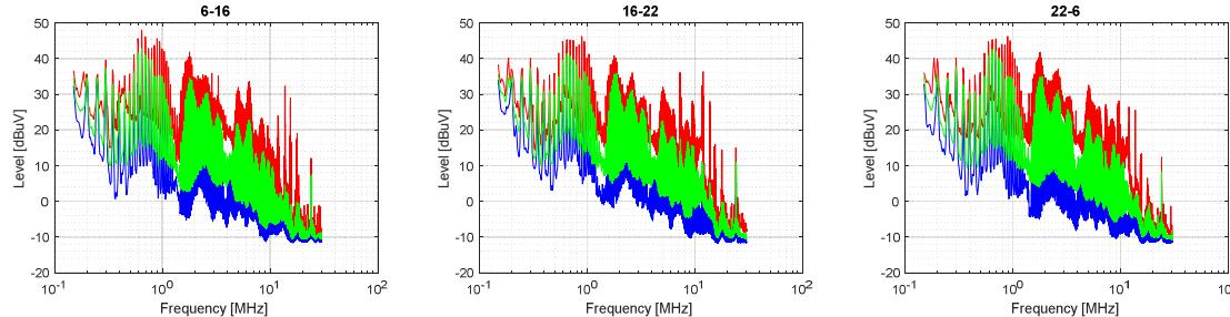
**Figure 4. Maximum (red), minimum (blue) and average (green) values for the conducted background noise level  $U_{n,b}$  measured in the 150 kHz – 30 MHz frequency range on all low voltage power lines:  $L_1$ ,  $L_2$ ,  $L_3$  and  $N$  for an urban area measured during the day (from 6 AM to 4 PM), the evening (from 4 PM to 10 PM) and during the night (from 10 PM to 6 AM)**
