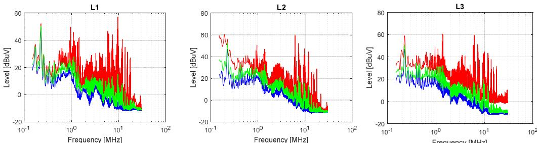
**Figure 5 Maximum (red), minimum (blue) and average (green) values for the conducted background noise level  $U_{n,b}$  measured in the 150 kHz – 30 MHz frequency range on each low voltage power line:  $L_1$ ,  $L_2$  and  $L_3$  in a rural area**
