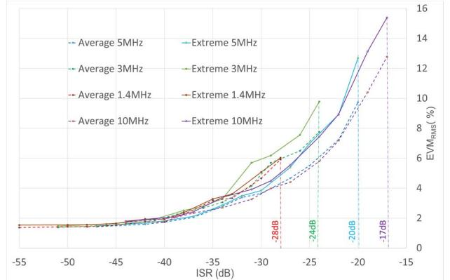
**Figure 5.** EVM as a function of the ISR, for a QPSK modulation.
