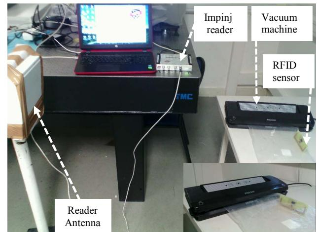
**Figure 4.** The View of the bench used during measuring absolute pressure and temperature.
