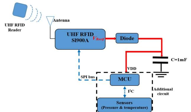
**Figure 1.** The block diagram of the proposed tag architecture
