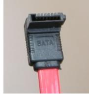
**Figure 1.** A seven-pin SATA data cable (left-angled version of the connector)
