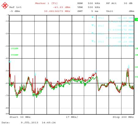
**Figure 4.** Radiated emission deriving from SATA interface while the transmission data is OFF (green color) and while transfer data is ON with 1 Gbit/s transmission speed (red color) in frequency range 30MHz – 200MHz
