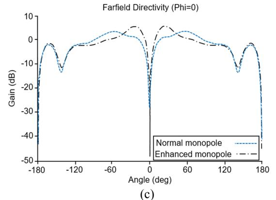
**Figure 3.** (a) Simulation results of  $|S_{11}|$ , (b) E-Plane radiation pattern of the proposed antenna at 2.8 GHz, (c) H-Plane radiation pattern of the proposed antenna at 2.8 GHz.
