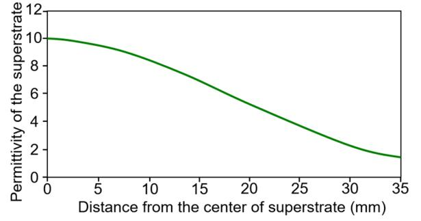
**Figure 2.** The ideal electric permittivity based on distance from center to have constant electric field phase.
