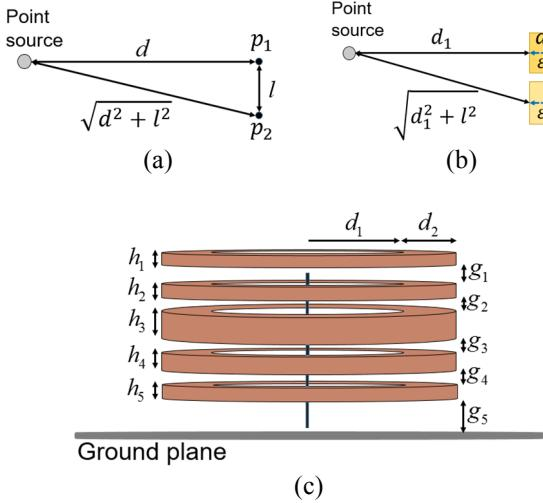
**Figure 1.** (a) Point source and phase difference between two points in a same plane, (b) adding dielectric layers around the point source, (c) overall view of the proposed enhanced gain monopole antenna.
